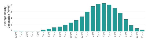
**Figure 2:** Average hourly generation from the Sun Peak Generating Station. The plant typically meets peak afternoon loads. It ran an average of 5.4 hours each time it started up between 2016 and 2018 and had a capacity factor of 1.3 percent. Batteries or solar+storage can serve a similar role on the grid.
